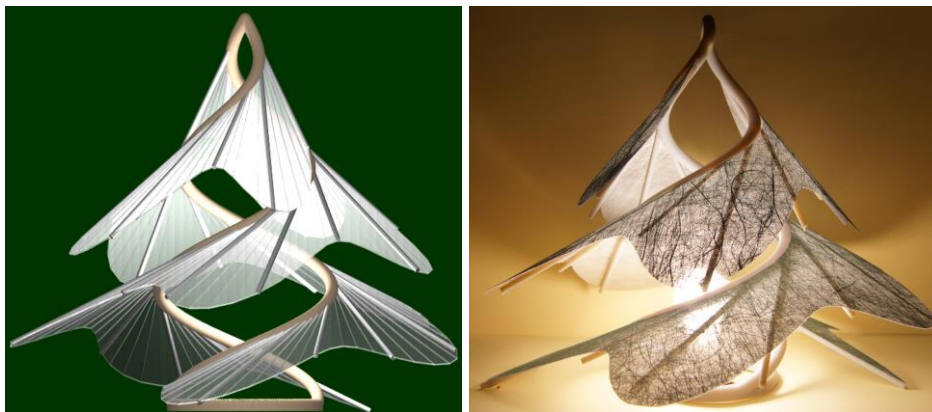
Figure 9 – The lampshade making use of tangent surface: designed image (left) and the fabricated model (right)
